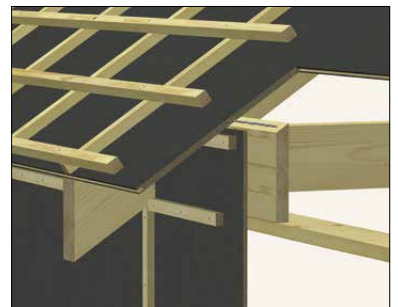
D10. Transition between wall and ceiling with loose protrusion
