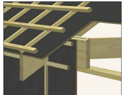
D9. Transition between wall and ceiling with protruding barrier
